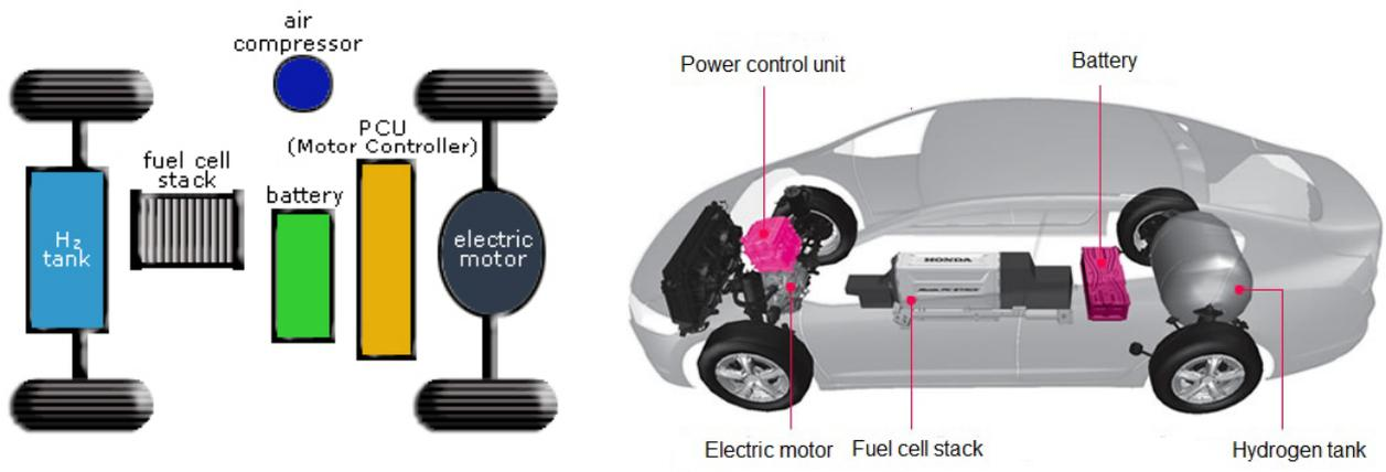
Figure 2: Schematic of a fuel cell vehicle [7]
