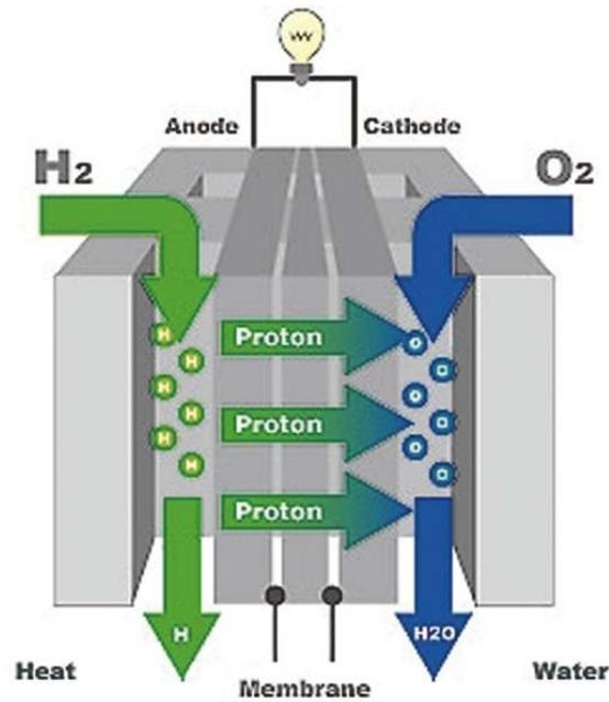
Figure 3: Technology of the fuel cell
